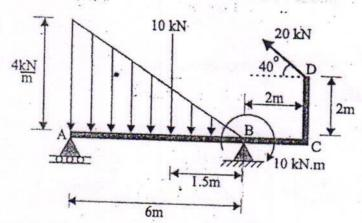
b) Determine the moment to be applied at C for equilibrium of pin jointed mechanism. Use virtual work method, Refer Fig. (06)
